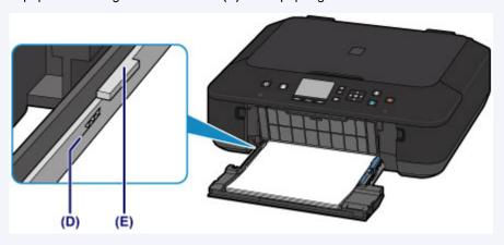
Load small size paper, such as 4" x 6" (10 x 15 cm), by pushing it in all the way to the back of the feeder.
