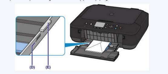
(6) Holding the right tab on the front tray, push the feeder back until the arrow (▶) on the front tray is aligned with the arrow (◄) on the machine.
