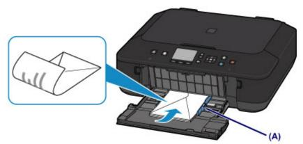
(5) Slide the right paper guide (A) to align the paper guides with both sides of the envelopes. Do not slide the paper guides too hard against the envelopes. The envelopes may not be fed properly.
