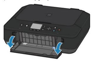
(2) Holding the right tab on the front tray, pull out the feeder until it stops.
